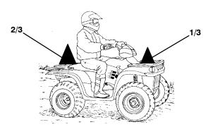
Your ATV has been designed to carry or tow a certain amount of load. Always read and understand the load distribution warning labels on the vehicle, and never exceed the weight capacities outlined in the specifications section of the owner's manual and on the safety decals.
